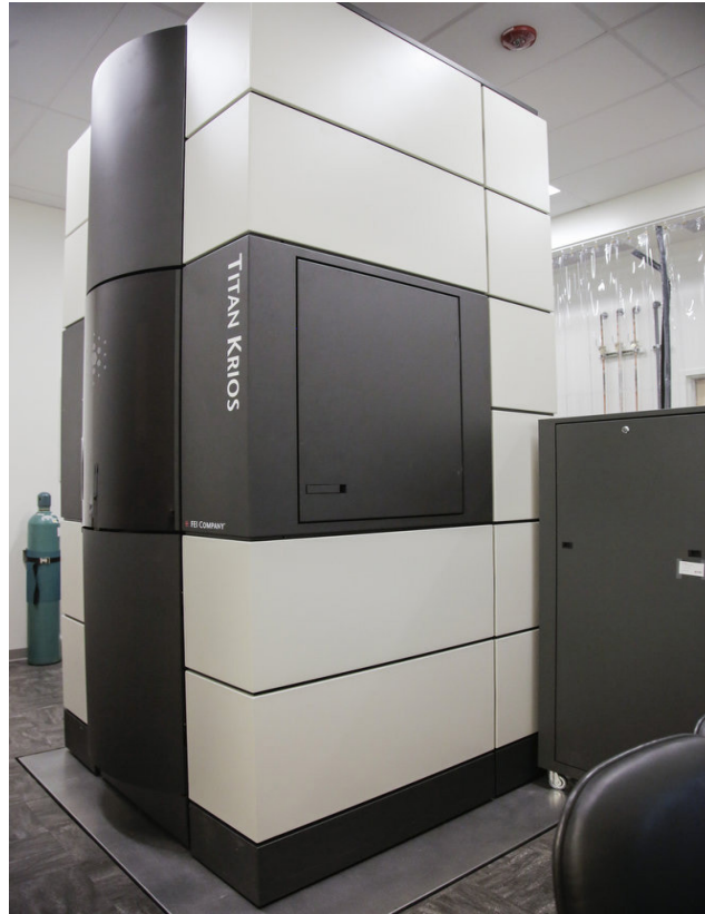
Figure 1: Typical set up of a Kryos TEM on a STACIS Quiet Island.
