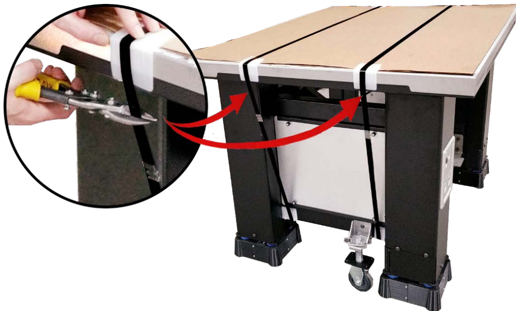
Figure 2-11 Remove protective top metal bands
