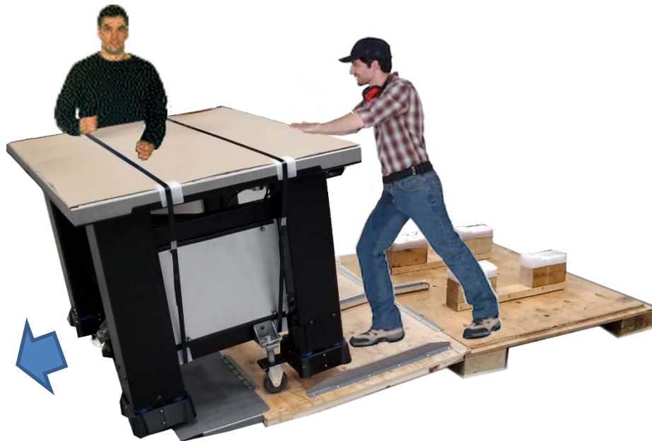
Figure 2-9 Roll system off platform
