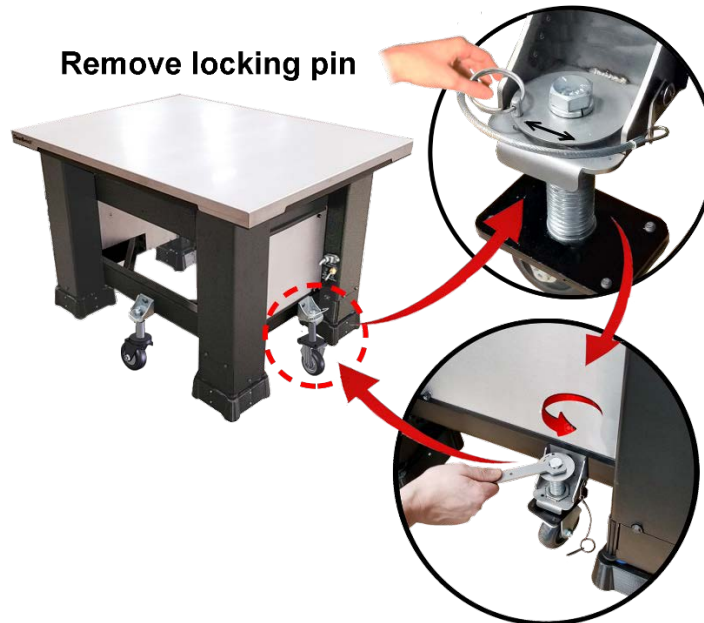
Figure 2-14 Rotate side casters 90 degrees toward narrow pathway
